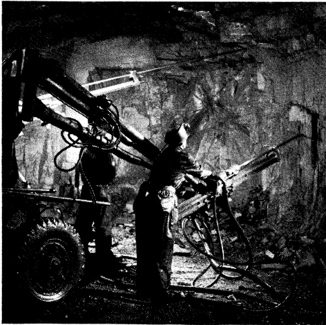
Extracting iron ore with electric drills at Wabana mine, under the ocean floor near Bell Island
